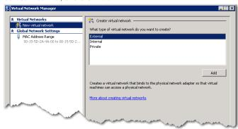
The New Virtual Network screen appears on the right. It defaults to an external interface, which also displays in the left column.
