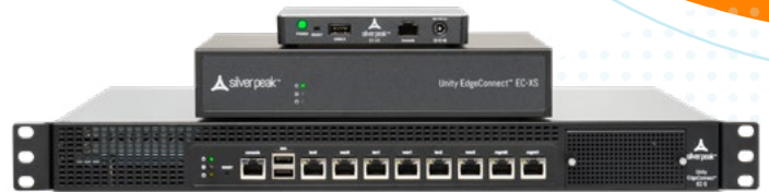
Figure 1: Aruba EdgeConnect physical appliances shown here are also available as virtual appliances.
