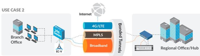
**USE CASE #2:** Small branch office security integrating Silver Peak EdgeConnect virtual appliances with Palo Alto Networks VM-Series firewall on a virtualized/universal CPE.
