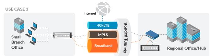
**USE CASE #3:** Small branch office security via backhaul to the remote (hub) firewall.
