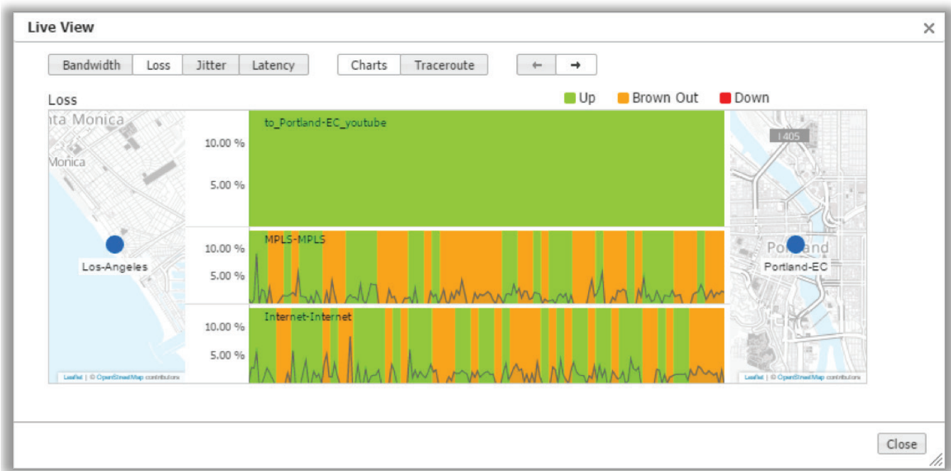
Figure 2: The Silver Peak LiveView window displays the benefits of combining tunnel bonding, FEC and business intent overlays to deliver an uninterrupted video stream shown in solid green, despite the packet loss (orange) shown in the underlying MPLS and internet links.
