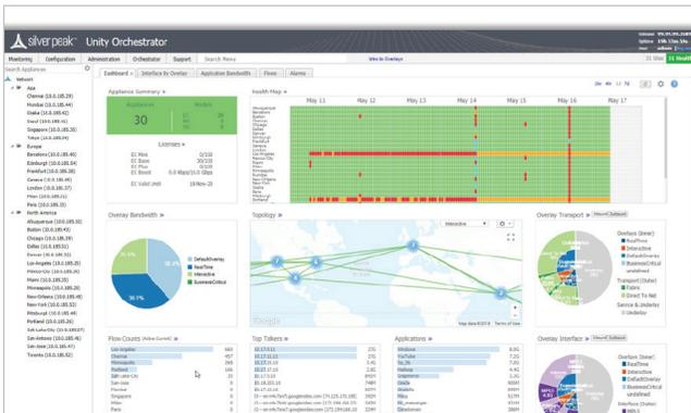
Figure 2: Orchestrator tenant dashboard provides status and details for each individual enterprise customer's SD-WAN deployment
