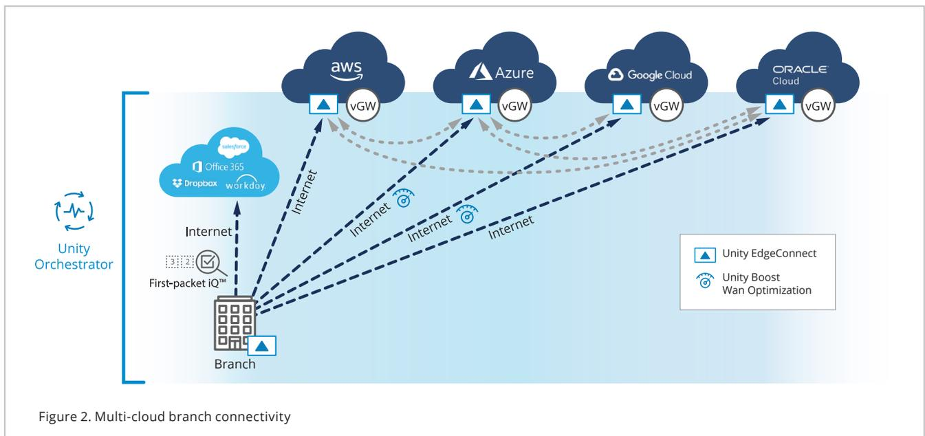
Figure 2. Multi-cloud branch connectivity
