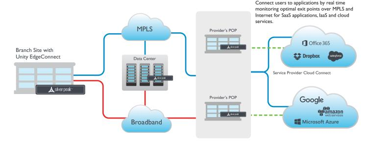
An EdgeConnectSP SD-WAN solution can enhance the performance of cloud-enabled applications. Both high and lower priority SaaS applications can be accommodated with either MPLS or broadband in this case.
