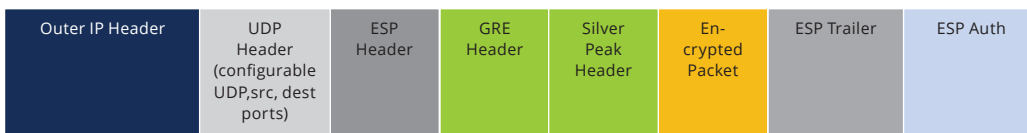
Figure 10: IPsec UDP (ESP) packet with Silver Peak encapsulation
